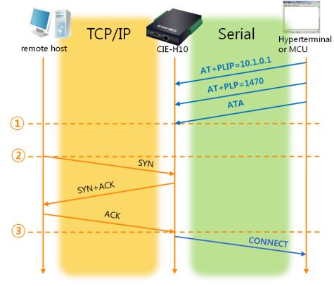
• TCP Server – setting parameters and a passive connection
