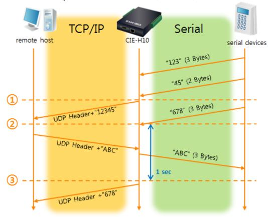
• Block Size: 5 bytes / Data Frame Interval: 1s (100 \* 10ms)
