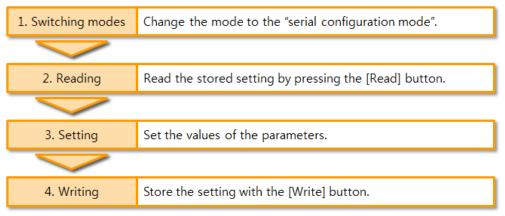
Figure 3-3 procedures for configuration via serial port
