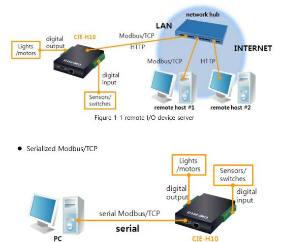
Figure 1-2 serialized Modbus/TCP
