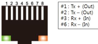
Figure 1-10 the RJ45 connector
