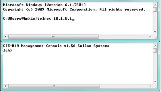
Figure 7-6 log in to CIE-H10 on TELNET
