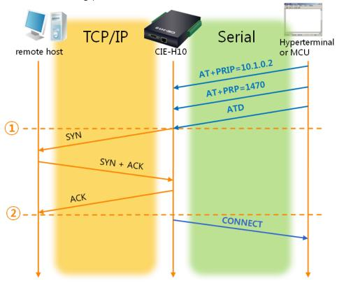
• TCP Client – setting parameters and an active connection
