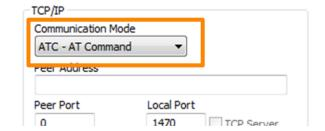
Figure 3-5 setting the communication mode to the AT command
