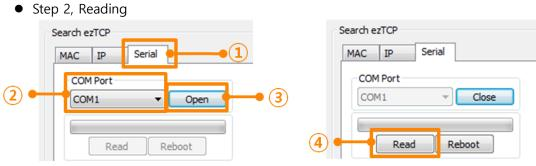
Figure 3-4 reading procedure via serial
