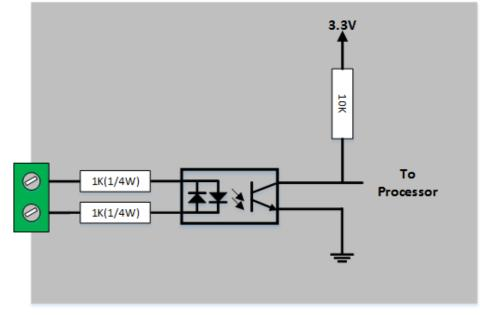
Figure 1-7 a circuit of the input port
