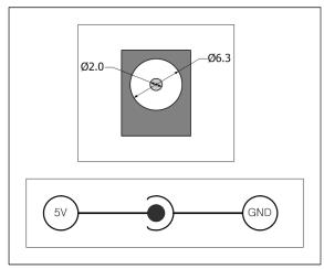
Figure 1-11 the power specification
