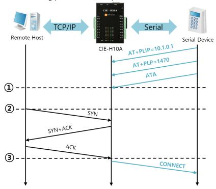
Figure 6-5 a passive TCP connection
