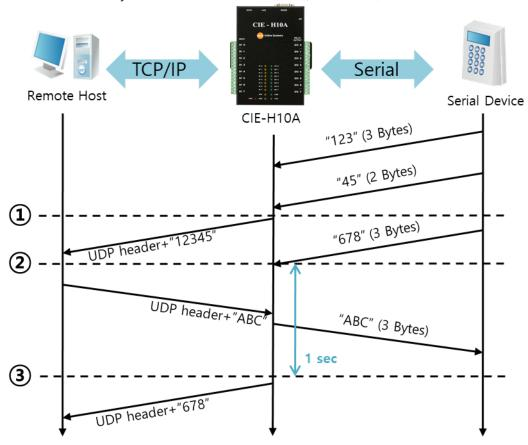
Figure 6-7 time chart for block size is 5 bytes and Data Frame Interval is 1s
