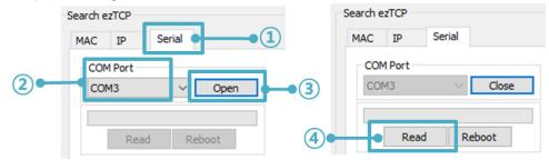
Figure 3-4 reading procedure via serial
