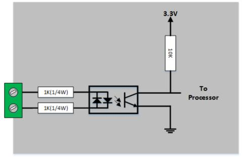
Figure 1-7 a circuit of the input port
