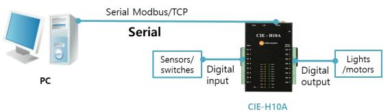
Figure 1-2 serialized Modbus/TCP
