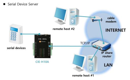
Figure 1-6 serial device server
