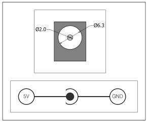
Figure 1-11 the power specification
