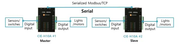
Figure 1-4 serial switch
