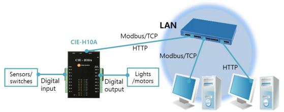
Figure 1-1 remote I/O device server
