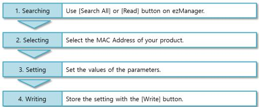
Figure 3-2 procedures for configuration via LAN
