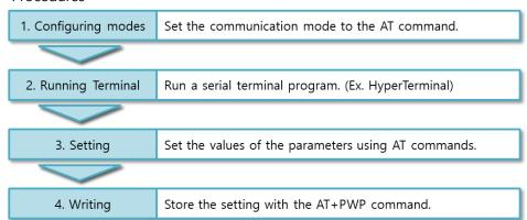
Figure 3-6 procedures for configuration with AT command
