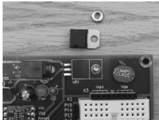
Figure C.1: Remove the 7805 regulator by cutting the leads close to the regulator case and unscrewing the small nut.
