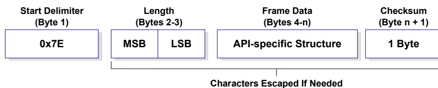
Figure 8-02. UART Data Frame Structure - with escape control characters:
