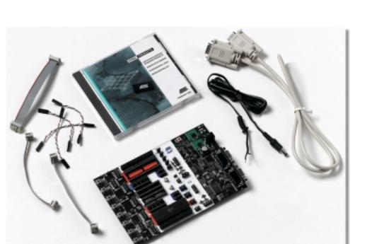
The Atmel AVR® STK500 is a starter kit and development system for Atmel's AVR Flash microcontrollers. The STK500 gives designers a quick start to develop code on the AVR combined with features for using the starter kit to develop prototypes and test new designs. The STK500 interfaces with AVR Studio®, Atmel's Integrated Development Environment (IDE) for code writing and debugging. The STK500 starter kit includes the following:
